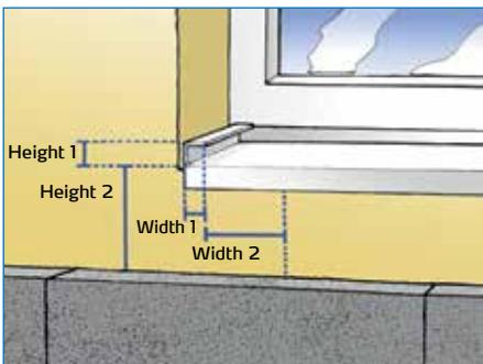
For making the cuts on windowsills, the processor of WDVS systems must take **four dimensions** on the facade in order to then transfer them to the plate to be fit.
