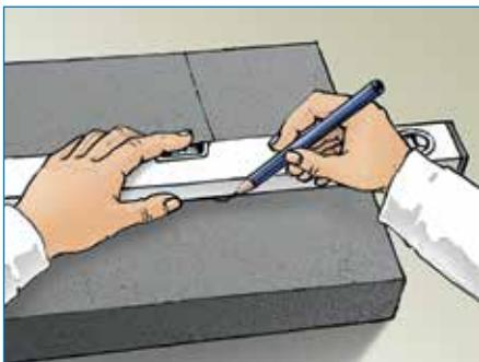
Extend the cut mark to the end of the plate.
