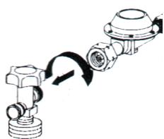
Connect the pressure controller to gas cylinder(s) or supply plant
