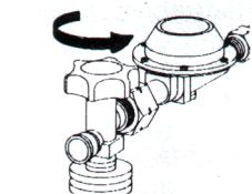
Open the cylinder valve(s) or stop valve of supply line. If gas is taken out of several gas cylinders simultaneously all the valves are to be opened.
