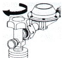
Close all the cylinder valves and stop valves of the supply line.
