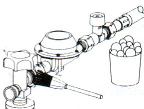
When the units have been installed and connected, all gas bearing connections are to be checked to ensure that they are tight (soap solution, leakage detection spray).
