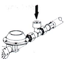
Press the unlocking button of hose shearing pin **after having opened** the valve(s).
